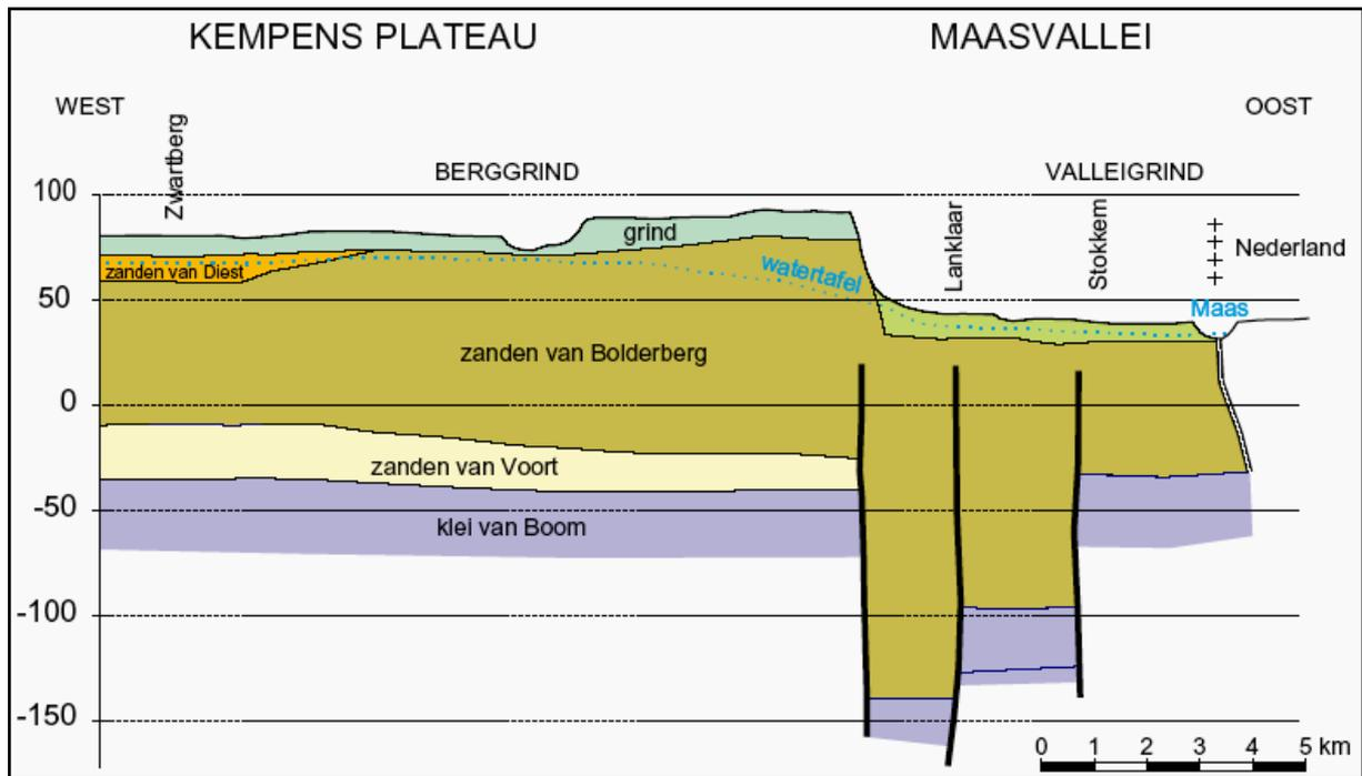
Fig.7. Geological WE-cross section from Zwartberg (Genk) to the Belgian-Dutch border, showing the topmost gravel layer, the layer-cake structure of the subsurface of the Campine Plateau and the fault-controlled steep eastern slope or escarpment ("steilrand")(Courtesy of ANRE, 1996)
